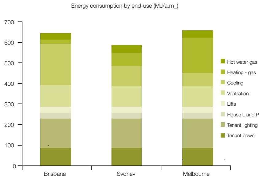
**Figure 7 – Office building energy consumption by end use**
