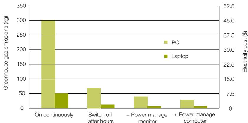
**Figure 11 – Annual greenhouse gas emissions and electricity consumption for PCs and laptops.**
